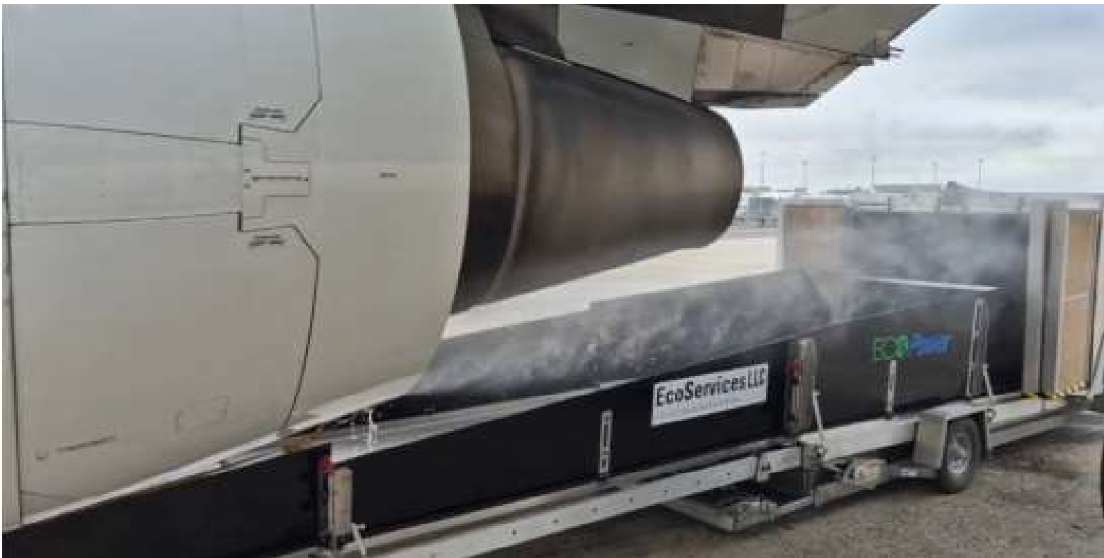
Cleaning of Amelia's CFM56 engines using ECOPower technology
